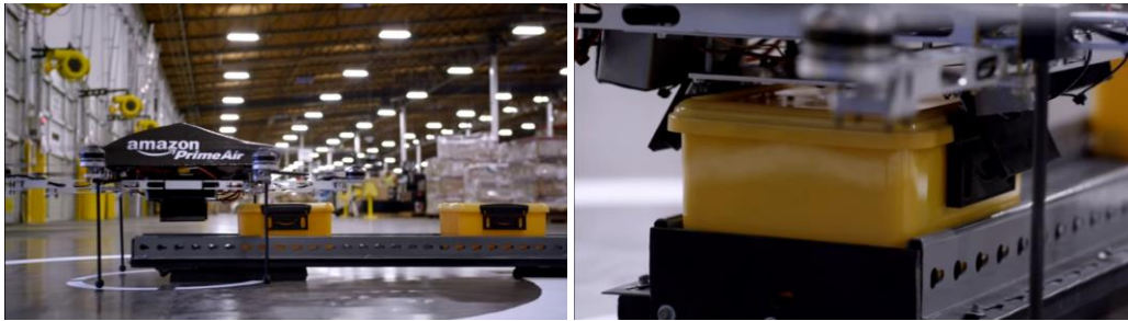
Figure 1: The 2013's depiction of the drones, from the side (left) and close up (right) as it prepares to clamp onto a package. The inner workings of the drone, such as its wires, are visible (right).
