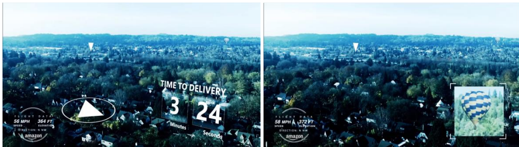
Figure 8: First-person view from the drone in horizontal flying mode. Flight data mimics that of an airplane. The drone identifies a hot air balloon in the sky as a potential hazard.
